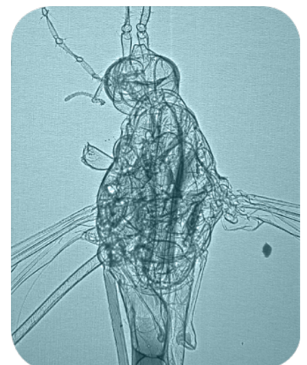
Detailed phase-contrast image of a fly from an all-optical laser driven betatron source
