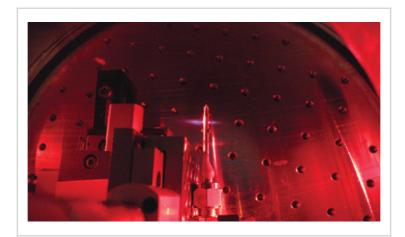
In a vacuum chamber, a quasi-static gas cell filled with neon triples the frequency of a broadband ultrafast IR-laser pulse. (Courtesy of Eleftherios Goulielmakis)
