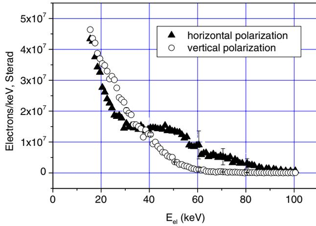
**FIGURE 2** Energy distributions of the electrons emitted by a fs-laser plasma for two perpendicular polarization directions. Horizontal polarization: E-field in the direction of observation. Vertical polarization: E-field perpendicular to the direction of observation
