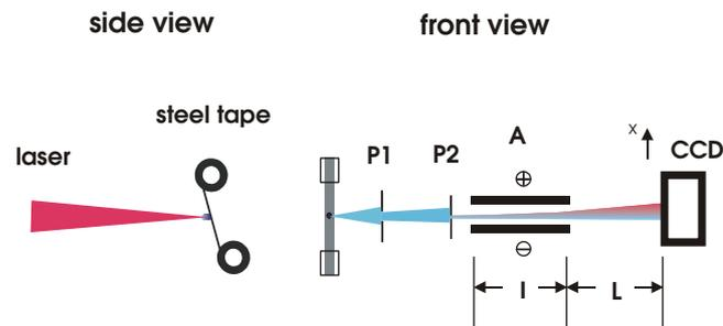
**FIGURE 1** Experimental arrangement for measuring the energy distribution of electrons laterally emitted from a fs-laser plasma. P1, P2: pinholes 1 mm and  $150 \mu\text{m}$  in diameter, respectively. A: electrostatic analyzer, plate length  $l = 5$  cm, plate separation 1 cm,  $L = 23$  cm. CCD: backside-illuminated X-ray CCD camera
