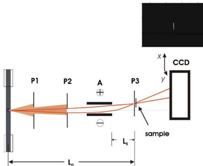
**FIGURE 3** Principle and realization of a time-of-flight electron streak camera. Pinhole P2 is opened to a diameter of 1 mm. Electrons of different energies propagate along different beam paths but coincide at the sample placed immediately behind pinhole P3.  $L_S = 16.5$  cm;  $L_0 = 53$  cm. The CCD image on top shows the streak recorded by the CCD with no sample behind P3
