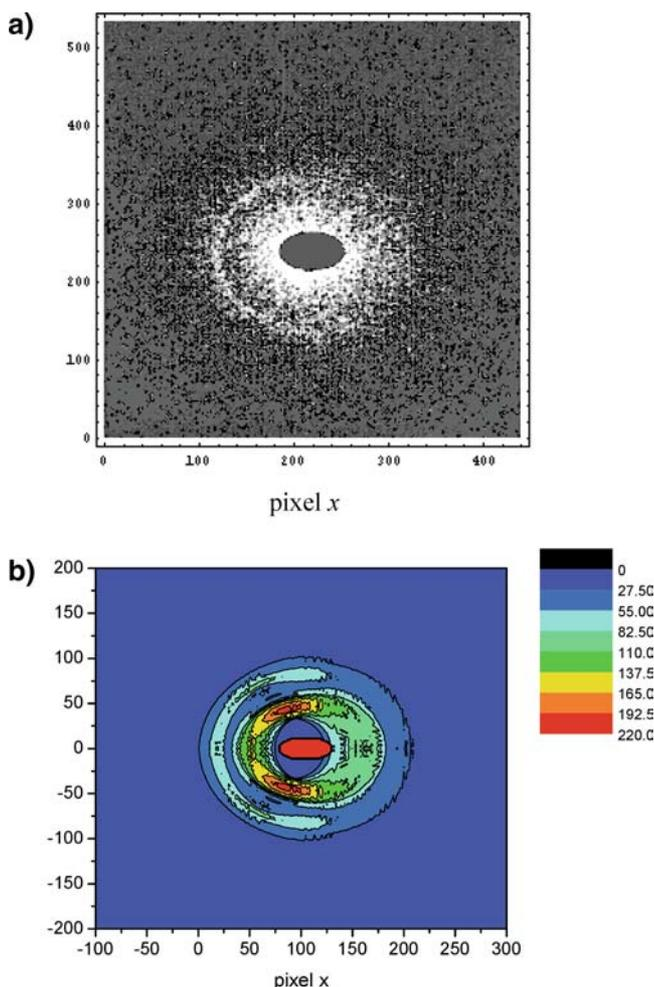
**FIGURE 4** **a** Streaked diffraction pattern from a thin aluminium sample, exhibiting characteristic asymmetry. Debye–Scherrer rings coincide on the left side, owing to their different radii; **b** Simulation of a streaked diffraction pattern under the conditions of the experiment. The asymmetry of the experimental pattern is reproduced. Here “pixel  $x$ ” corresponds to the vertical direction of the CCD
