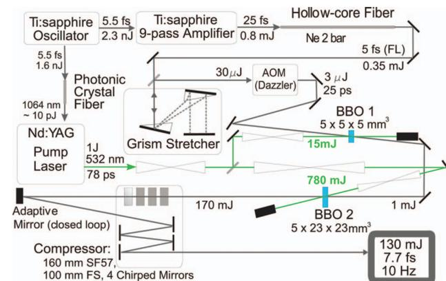
Fig. 1. Schematic layout of the NOPCPA setup.
