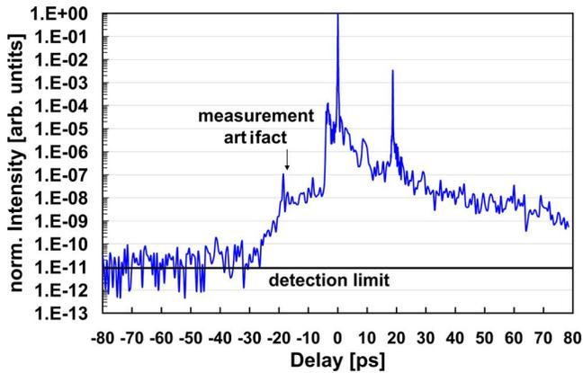
Fig. 4. (Color online) Third-order autocorrelation (negative delays correspond to the pulse leading edge): contrast of the amplified and compressed pulse; the peak at  $-18.8$  ps is a measurement artifact belonging to the corresponding postpulse, and contributions for  $t < -30$  ps are background noise.
